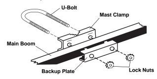
3. Attach the other mast clamp assembly to the cradle boom. (Be sure it faces the same direction as the main boom's mast clamp assembly, shown above.) Fold out the two sets of metal support straps on the cradle boom and attach them to the corresponding holes on the main boom using the two supplied 11/2-inch screws and large wing nuts.
